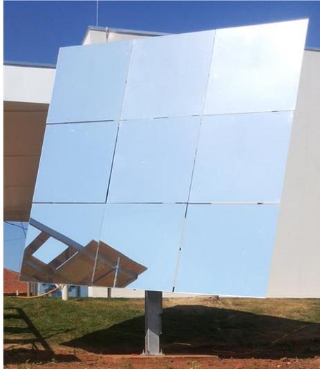
Figure 8: Prototype of the 9 m<sup>2</sup> heliostat being employed in the SMILE project pilot plants.
